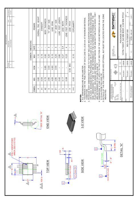
Figure 1 EMC1152 10-Pin MSOP Package Drawing
